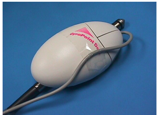
Figure 2: FieldMouse#2: Combination of a barcode reader and a gyro-mouse.
