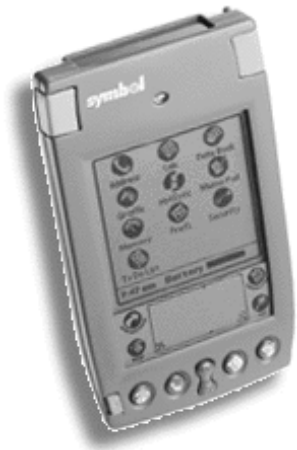
Figure 3: FieldMouse#3: PalmIII PDA including a laser scanner and a tilt sensor.
