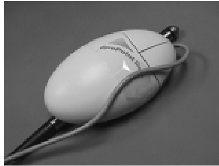
Fig. 2. FieldMouse#2: Combination of a barcode reader and a gyro-mouse.
