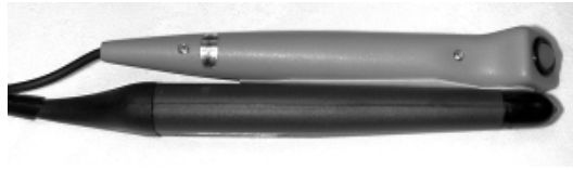
Fig. 1. FieldMouse#1: Combination of a barcode reader and a pen-mouse.
