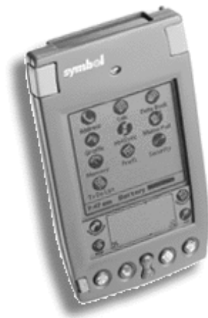
Fig. 3. FieldMouse#3: PalmIII PDA including a laser scanner and a tilt sensor inside.
